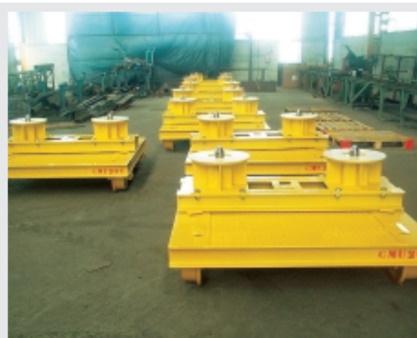
Bogie remorque, 1900 mm, voie 1440 mm, charge 20 t Trailer bogie 20 t, 1900 mm, gauge 1440, load 20 t
