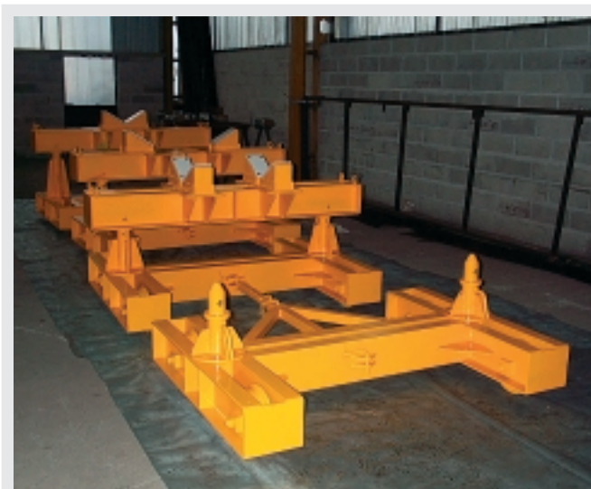
Ensemble de chariot manuel 4 m x 2 m - transport de rotor - charge 10 t Manual truck for rotor 4 m x 2 m - load 10 t
