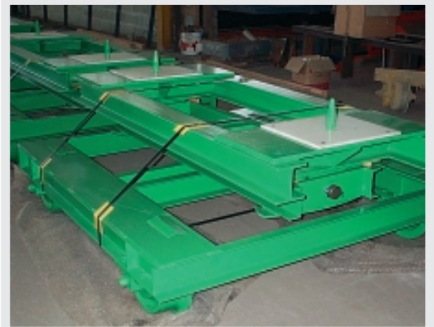
Chariot manuel à double rotations 1 horizontale 1 verticale, charge 10 t Truck with double rotation vertical and horizontal plane, load 10 t
