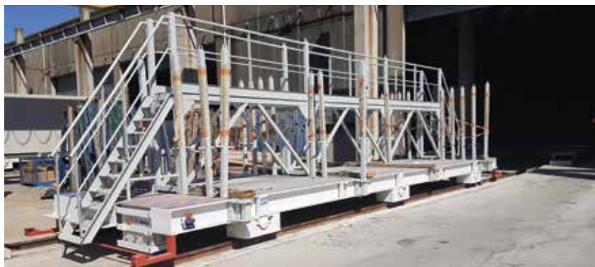
Chariot porte dalles béton motorisé 100 T Electrical powered trolley with racks (ex : for concrete block handling), load 100 T
