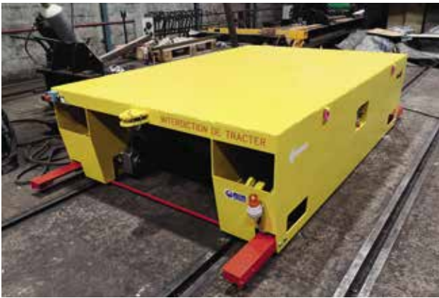
Chariot motorisé sur batteries 10 T Electrical powered trolley on batteries, load 10 T
