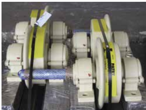
Roues entre paliers 97-3 motorisable 400 M Wheels 400 M between bearers with 97-3 assembly (axle adjustable to engine)
