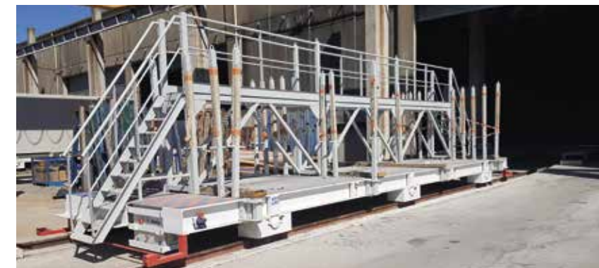
Chariot porte dalles béton motorisé 100 T Electric powered trolley with racks (ex : for concrete block handling), load 100 T
