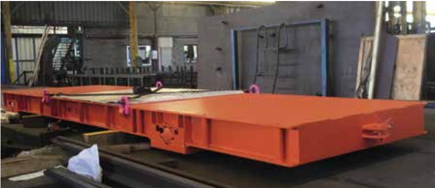
Chariot manuel 25 T Manual trolley, load 25 T
