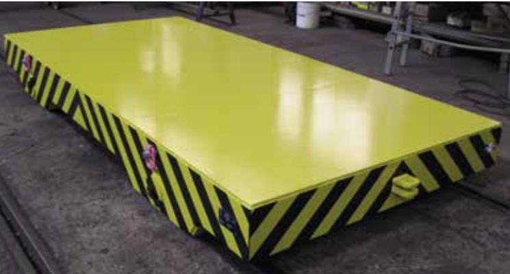
Chariot manuel 30 T Manual trolley, load 30 T
