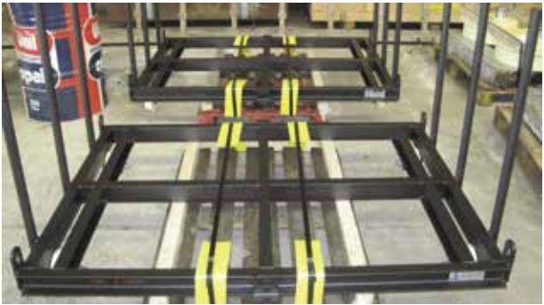
Chariot manuel 2 T Manual trolley, load 2 T
