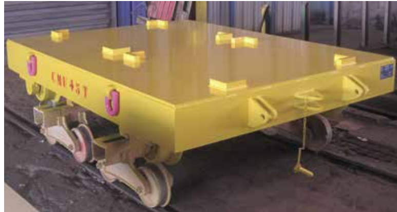
Chariot manuel 45 T Manual trolley, load 45 T
