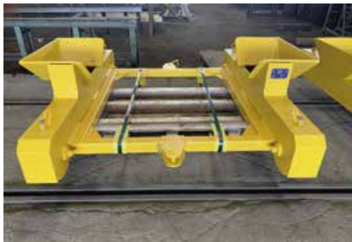
Chariot manuel 8 T Manual trolley, load 8 T
