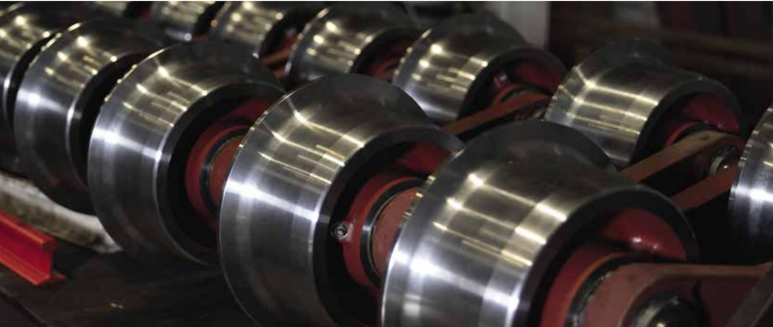
Ensemble de 2 roues 100 x 85 montées entre flasques D11 Set of 2 wheels 100 x 85 mounted between D11 flanges
