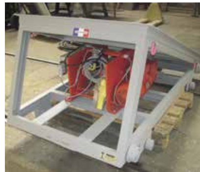
Chariot manuel 1 T Manual trolley, load 1 T
