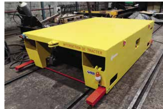
Chariot motorisé sur batteries 10 T Electric powered trolley on batteries, load 10 T
