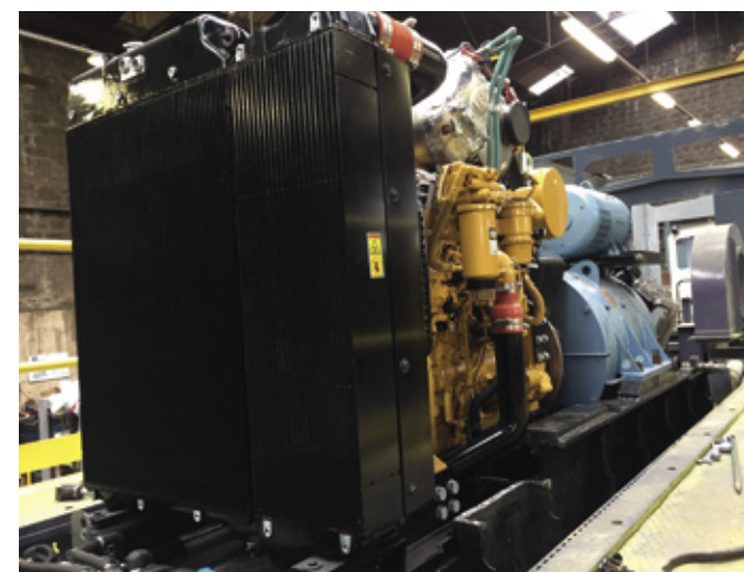
Remotorisation en CATERPILAR C9.3B de 340 kW Remotorization with Caterpillar C9.3B motor
