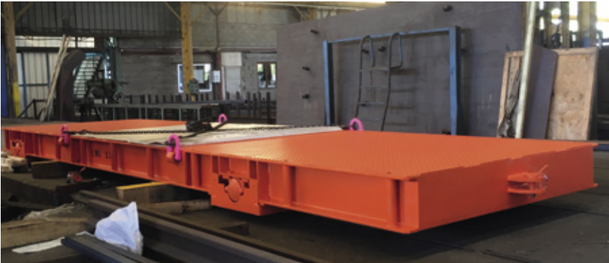
Chariot manuel 25 T Manual trolley, load 25 T
