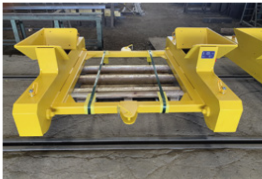
Chariot manuel 8 T Manual trolley, load 8 T
