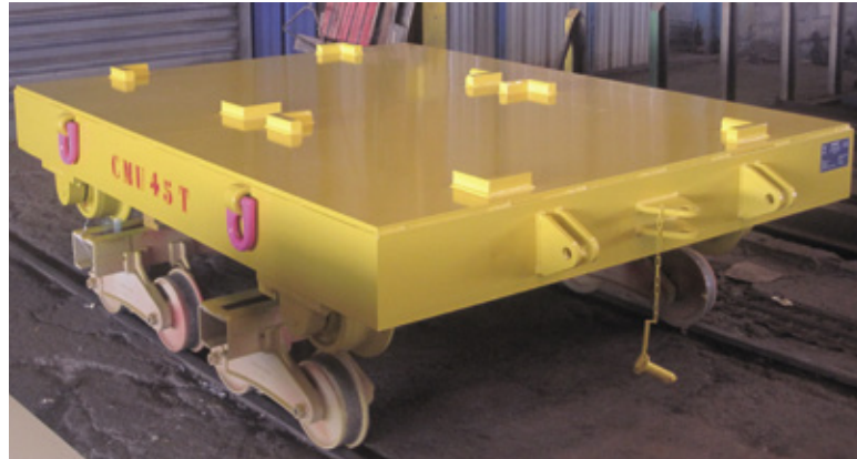
Chariot manuel 45 T Manual trolley, load 45 T
