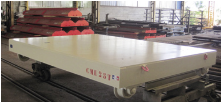
Chariot manuel 25 T Manual trolley, load 25 T
