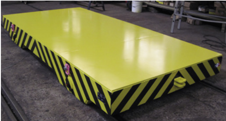
Chariot manuel 30 T Manual trolley, load 30 T
