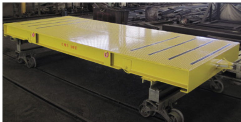
Chariot manuel 18 T Manual trolley, load 18 T
