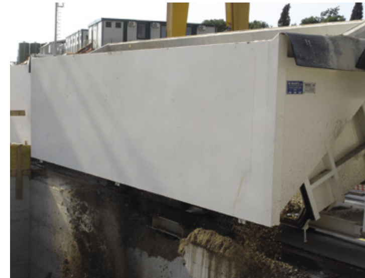
Berline basculante Side discharge muck car
